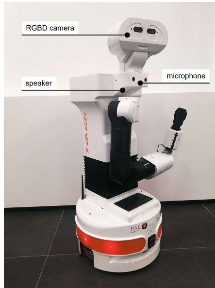
Fig. 2. TIAGo, the service robot used to test the proposed framework. The locations of the onboard sensors used for HRI are highlighted.
