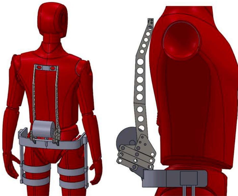
Fig. 1. Active adaptive back-support exoskeleton with backbone-based kinematics.
