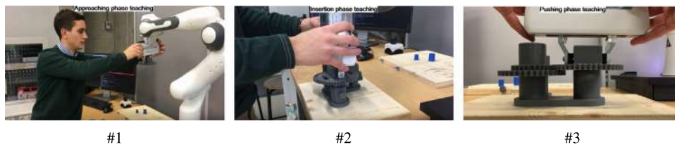
Fig. 7. HMM algorithm applied to the learning of the three subtasks: approaching subtask #1, insertion subtask #2, pushing subtask #3.
