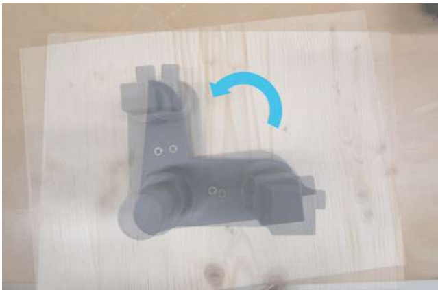
Fig. 8. Simulated task assembly location pose uncertainties for the evaluation of the BO algorithm capabilities.
