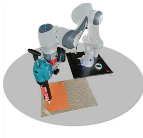
Fig. 1: Experimental setup for the validation of the proposed user's pairwise preferences-based optimization methodology applied to the tuning of a velocity planner for the execution of a sealing task. A Franka EMIKA panda robot is equipped with a MAKITA sealing gun. A servomotor (controlled with Arduino) has been embedded in the ad hoc designed flange to activate/deactivate the deposition.
