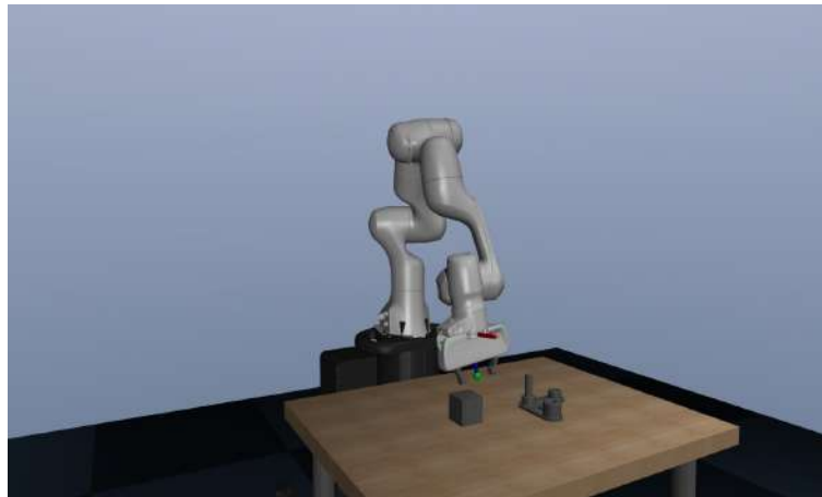
Figure 4. Franka EMIKA panda robot employed in the target grasping task in the MuJoCo environment.
