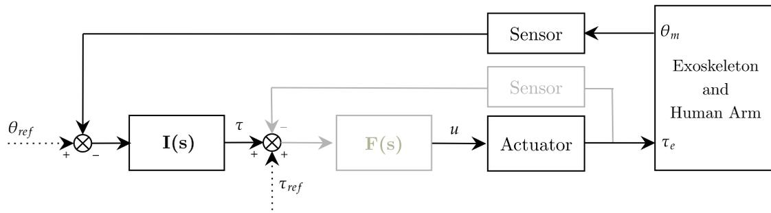
**Figure 3.** Impedance control scheme in the joint-space. Implicit (black) and explicit (black and gray).  $I(s)$  is the impedance controller,  $F(s)$  is the force controller (only explicit).  $\theta_{ref}$  and  $\tau_{ref}$  represent respectively reference angular position and torque, while  $u$  refers to the motor current control signal.
