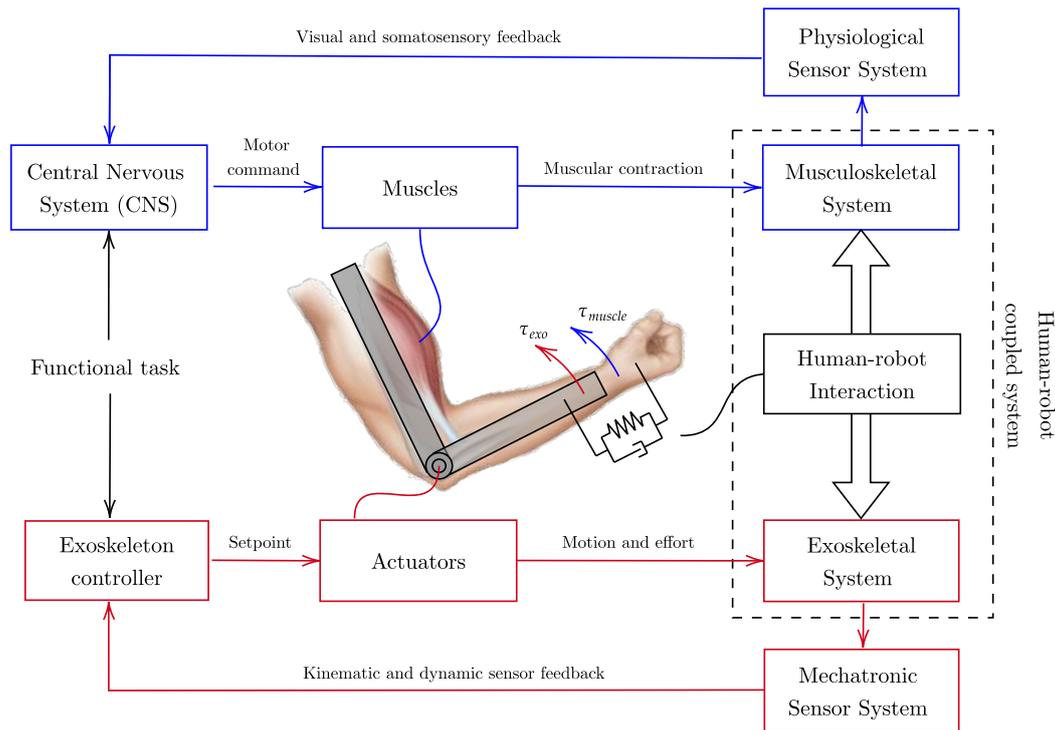
**Figure 1.** Human-robot interaction representation. The blue scheme represents human motor control, and the red scheme refers to the exoskeleton control. The human-robot coupled system cooperates towards the completion of a shared functional task.
