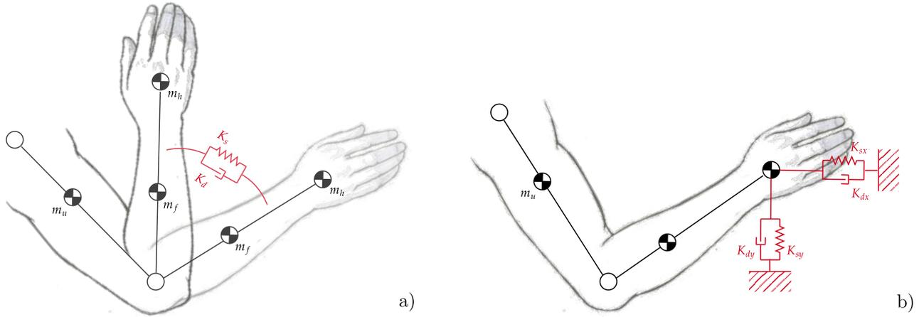
**Figure 4.** (a) First order impedance model applied at the elbow joint in the joint-space. (b) First order impedance model applied at the elbow joint in the Cartesian-space.
