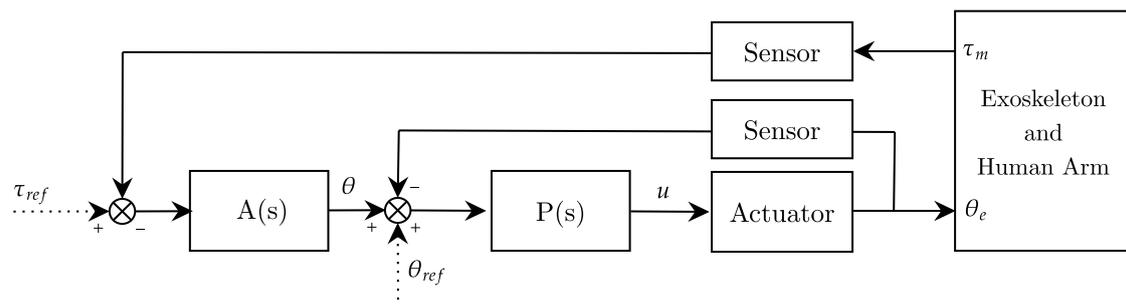
**Figure 6.** Admittance control scheme in the joint-space.  $A(s)$  is the admittance controller,  $P(s)$  is the position controller.  $\theta_{ref}$  and  $\tau_{ref}$  represent respectively reference angular position and torque, while  $u$  refers to the motor current control signal.
