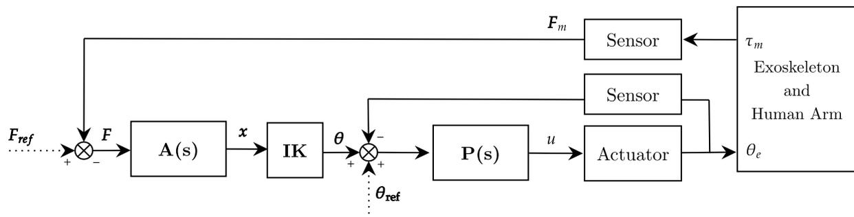
**Figure 7.** Admittance control scheme in the task-space.  $A(s)$  is the task-space admittance controller,  $P(s)$  is the joint-space position controller.  $IK$  corresponds to the inverse-kinematics algorithm.  $\theta_{ref}$  and  $\tau_{ref}$  represent respectively reference angular position and torque, while  $u$  refers to the motor current control signal.
