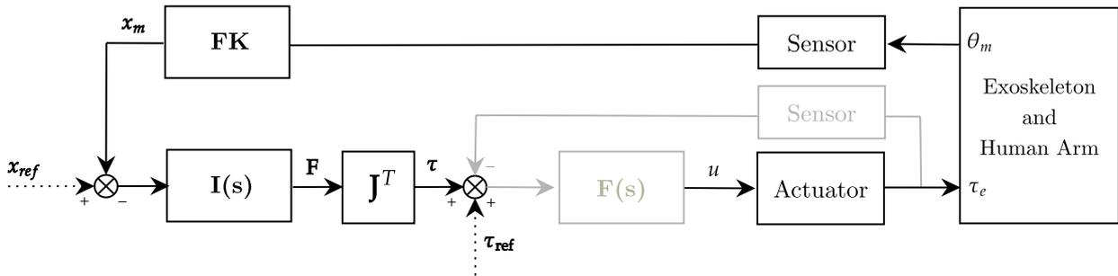
**Figure 5.** Impedance control scheme in the Cartesian-space. Implicit (black) and explicit (black and gray).  $I(s)$  is the impedance controller,  $F(s)$  is the force controller (only explicit).  $FK$  represents the forward kinematics model of the exoskeleton, and  $J^T$  corresponds to the transposed Jacobian matrix.  $\theta_{ref}$  and  $\tau_{ref}$  represent respectively reference angular position and torque, while  $u$  refers to the motor current control signal.
