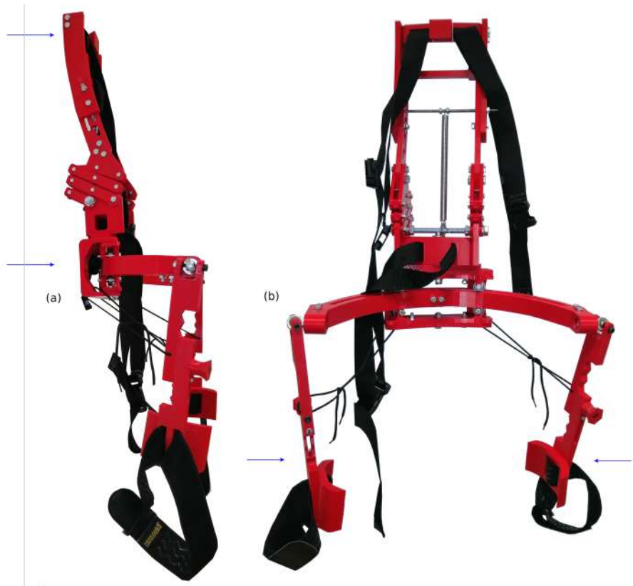
Fig. 1: Our low-back exoskeleton featuring the backbone-tracking kinematic structure (a) and passive actuation (b). WSU position is shown with blue arrows.
