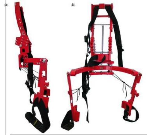
Fig. 1. Low-back exoskeleton prototype with backbone-tracking kinematics (a) and passive actuation (b).
