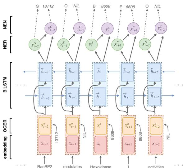
Figure 3: Architecture of the BiLSTM-based sequence tagger (simplified).
